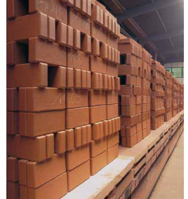
Fired clinker pavers after they have exited the kiln
