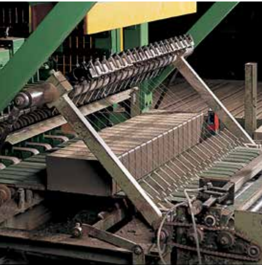
The clay column is divided by a harp-wire cutter into the paver sizes
