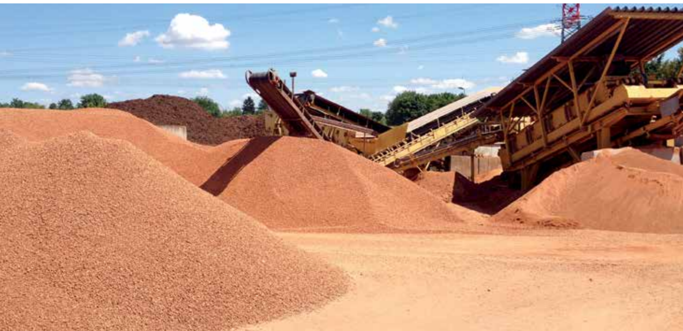
Production of recycled aggregates for use as substrate in vegetation engineering.
