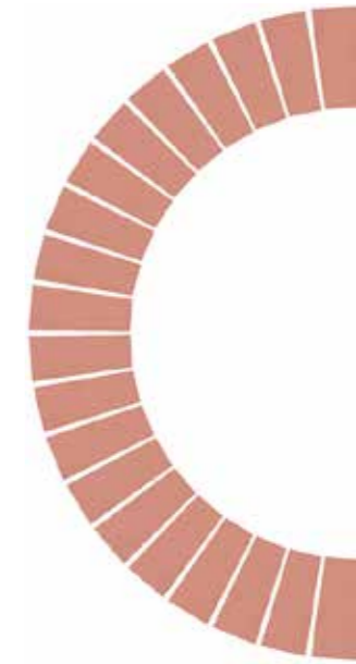
Fig. A5-7: Tree ring with wedge-shaped clinker pavers
