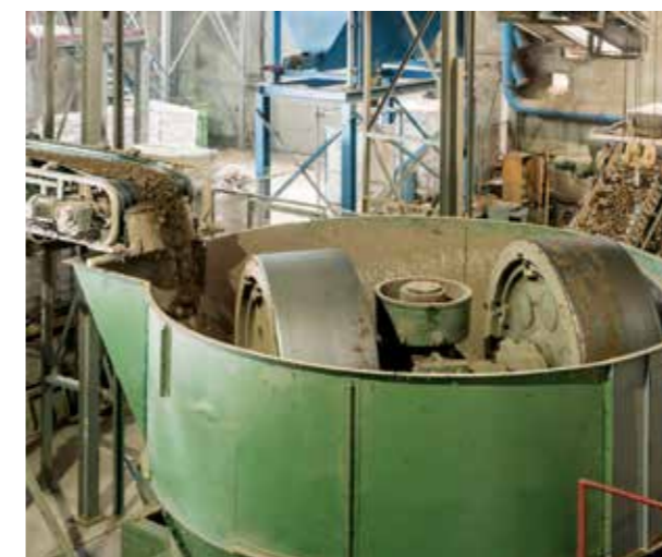
Pan mill, two heavy rollers comminute the clay
