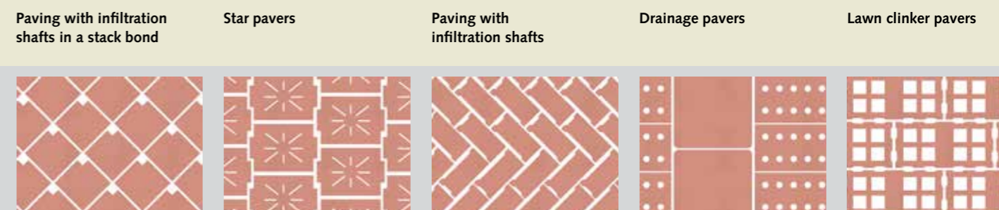
Fig. 6-3: Different clinker paver formats for permeable paving
